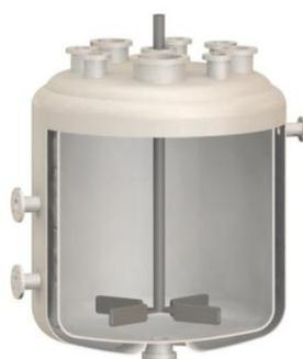
**Figure 1:** Batch reactor with single external cooling jacket
