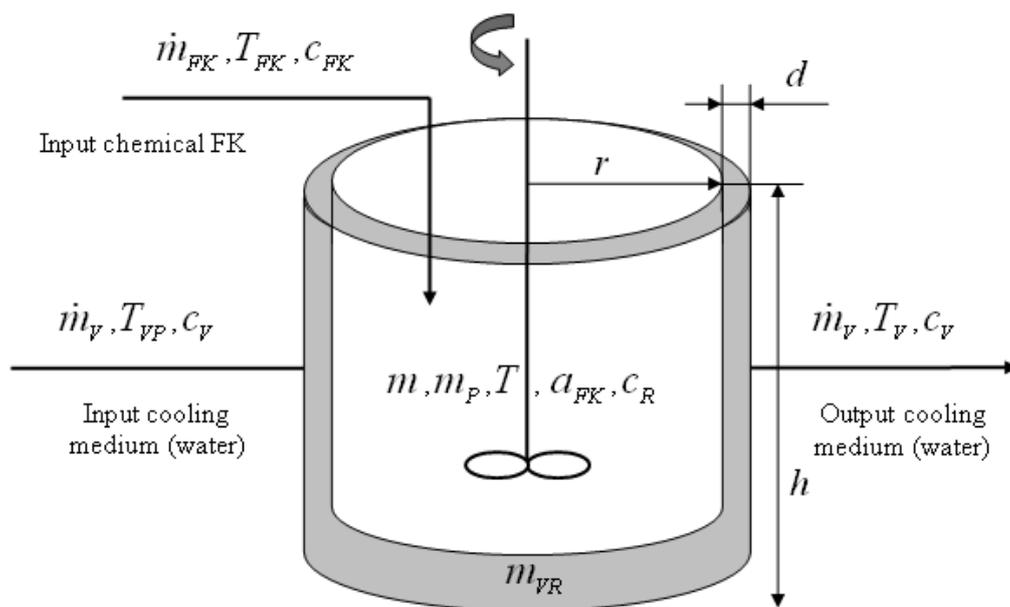
**Figure 2: Batch reactor**
