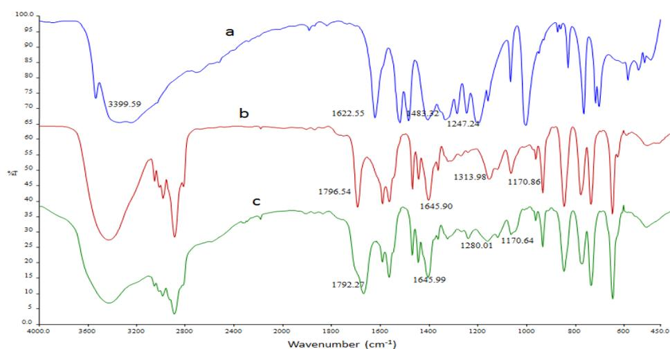
**Figure 2:** FTIR spectra for (a) Pyrogallol (Py); (b) Pyrogallol-Imprinted Polymer (PIP) and (c) Non-Imprinted Polymer (NIP)
