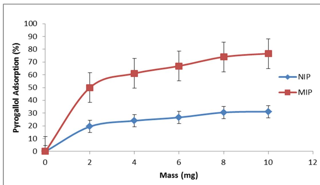
**Figure 3:** Pyrogallol adsorption of pyrogallol from pyrogallol solution by Non-Imprinted Polymer (NIP) and Pyrogallol-Imprinted Polymer (PIP)
