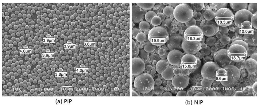
**Figure 1:** SEM Images of (a) PIP and (b) NIP
