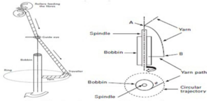
Figure 4: S-twisted model on Ring Spinning
