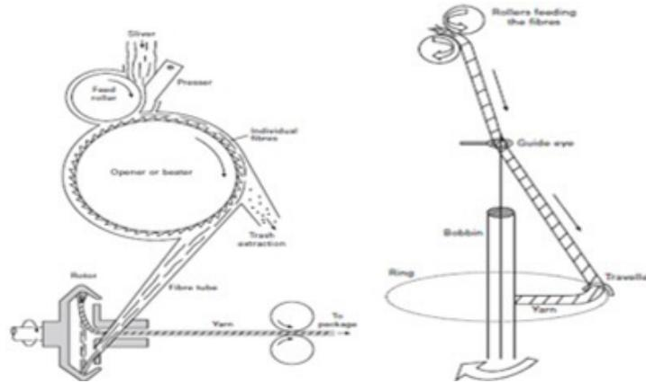
Figure 1: Movement of Yarn inside Open End Rotor Spinning and Ring Spinning.
