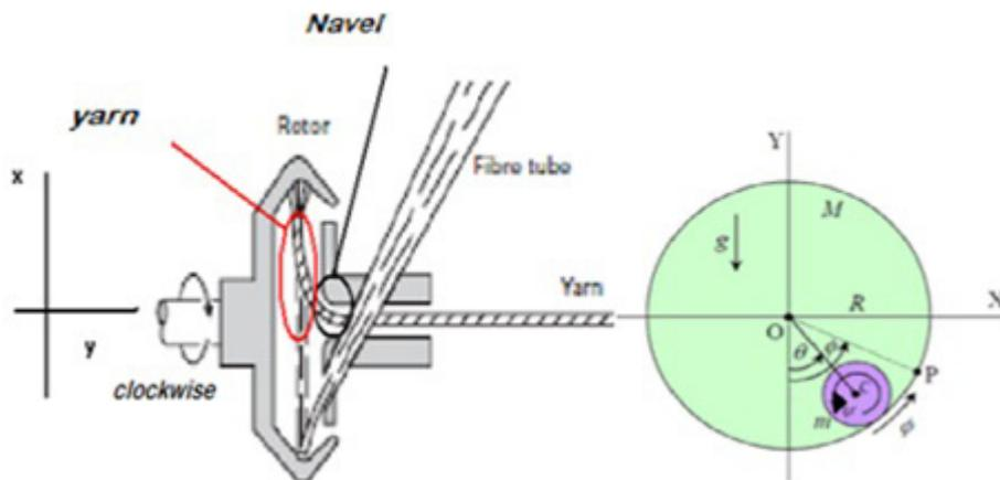
Figure 5: S-twisted model on Rotor Spinning
