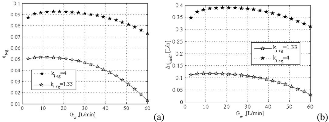
**Fig.6. Influence of volume flow rate of water  $G_w$ : (a) – on TEG efficiency  $\eta_{\text{teg}}$ , (b) – on fuel consumption reduction  $\Delta q_{\text{fuel}}$**
