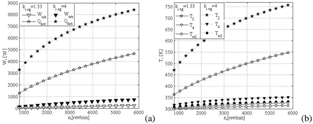
**Fig.2. Influence of IC-engine shaft rotation speed  $n_E$  (a) – on TEG power  $W_{teg}$  and supplied thermal flow  $Q_{hot}$ , (b) – on specific temperatures**
