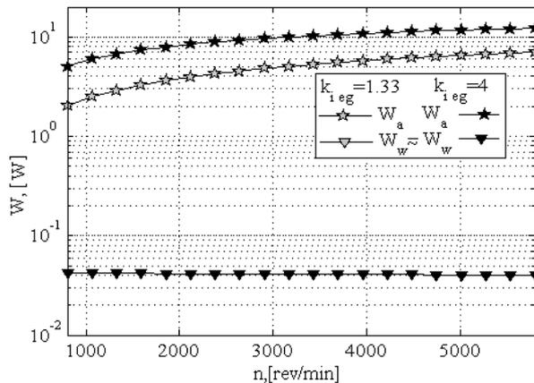
**Fig.3. Influence of IC-engine shaft rotation speed  $n_E$  on electrical consumption of the TEG components: hydraulic losses  $W_w$  and losses on ventilator operation  $W_a$**
