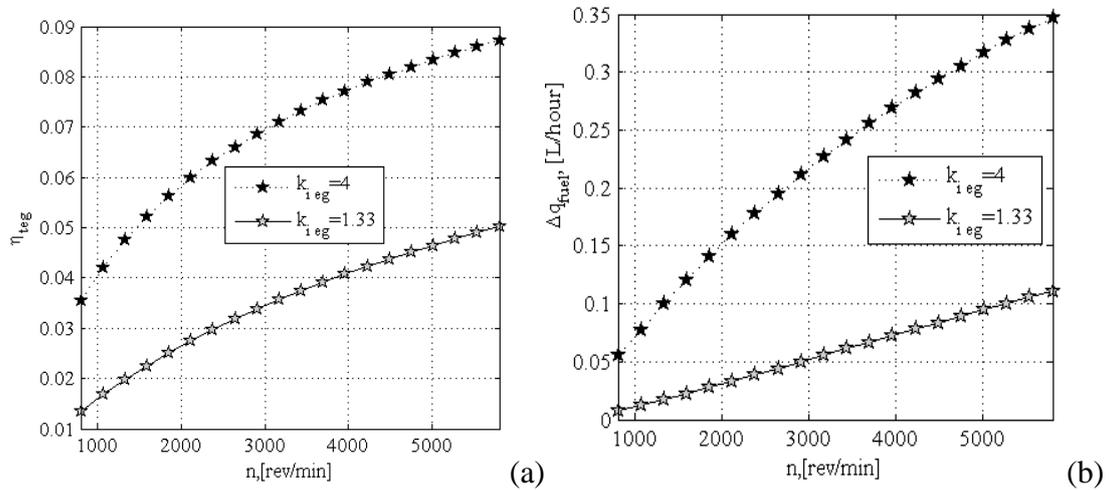
**Fig.4. Influence of IC-engine shaft rotation speed  $n_E$ : (a) – on TEG efficiency; (b) – on fuel consumption reduction  $\Delta q_{fuel}$**
