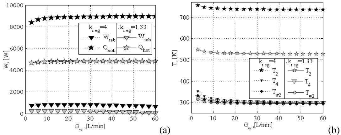
**Fig.5. Influence of volume flow rate of water  $G_w$ : (a) – on the TEG power  $W_{teg}$  and passing through it thermal flow  $Q_{hot}$ ; (b) – on specified temperatures**
