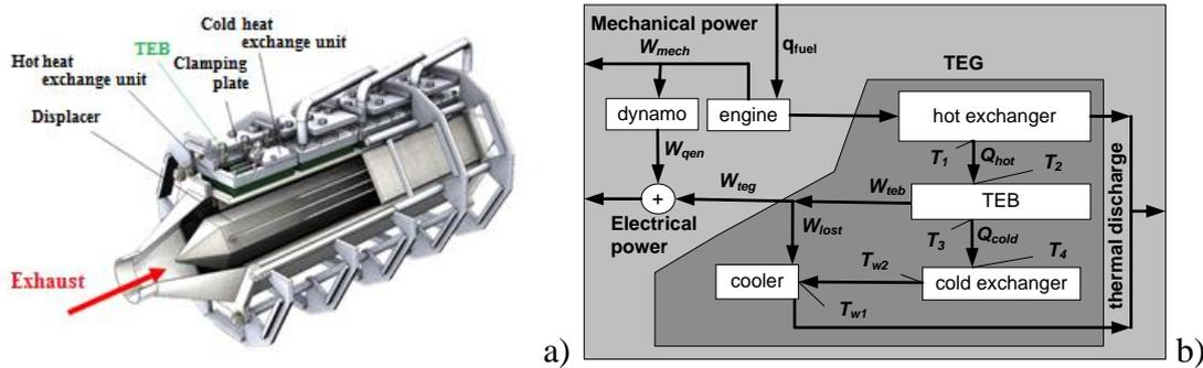
**Fig.1. TEG schematic: a) – heat-exchange unit, b) – flowchart**
