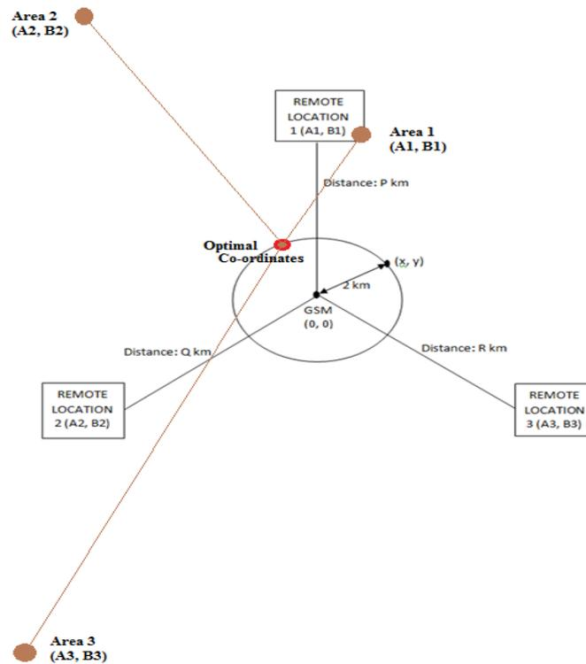
**Figure 3:** Optimal Placement of Zigbee using Genetic Algorithm (GA)
