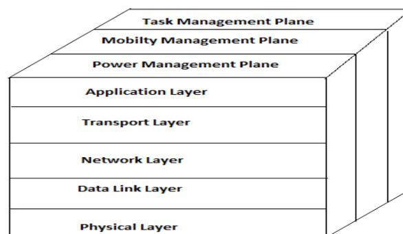
**Figure 3:** Protocol stack used by sensor node
