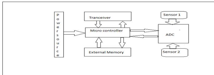
**Figure 2:** Architecture of sensor node
