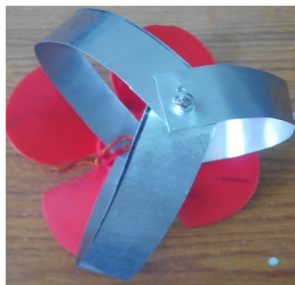
Figure 2: The special designed wind turbine consisting of vertical wind turbine mounted over propeller.
