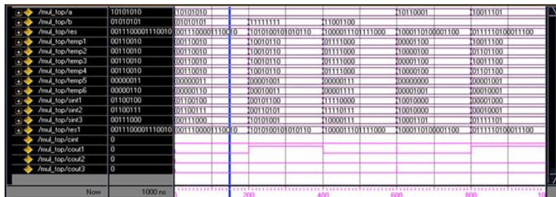
Figure 5: Simulation result for 8×8 Vedic multiplier using Urdhva Tiryagbhyam Sutra.
