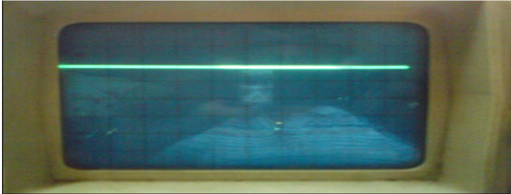
Figure 5f: Rectifier output voltage waveform.
