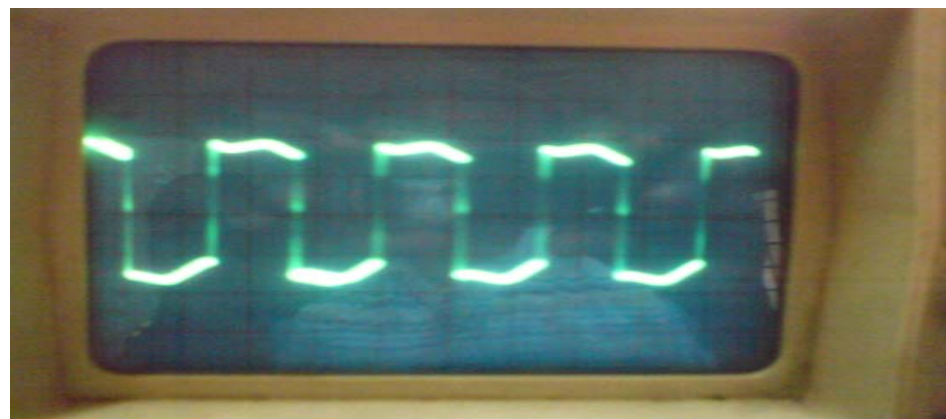
Figure 5e: Output voltage of Push pull converter.
