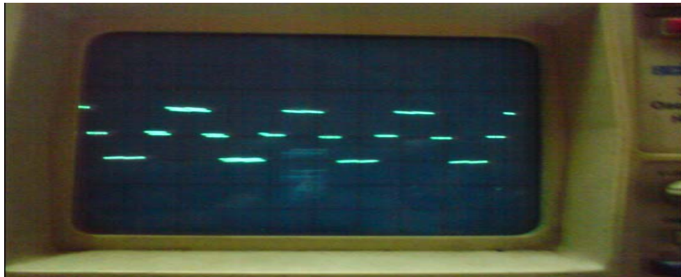
Figure 5g: Phase voltage of three phase inverter.
