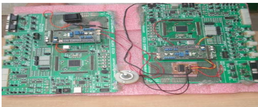
Figure 8: Interfacing ECU and electric window node.
