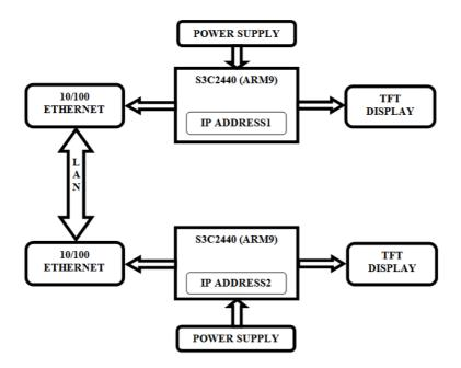
This project contains ARM9 board which is having in built memory where we store program. The ARM9 board uses a 1.8v power supply.
