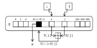
The lookup stage of RC4. The output byte is selected by looking up the values of S(i) and S(j), adding them together modulo 256, and then using the sum as an index into S; S(S(i) + S(j)) is used as a byte of the key stream, K.
