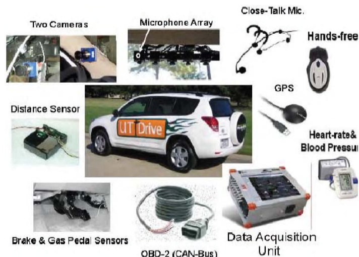
Figure 1: Data collection vehicle and incorporated sensors.
