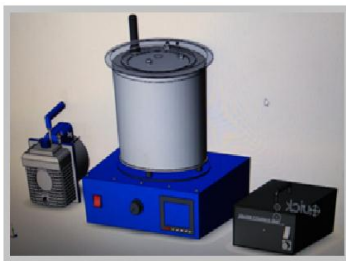
Figure 3: Construction of Modified spin coater
