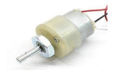
A small motor (ac induction, permanent magnet dc, or brushless dc) designed specifically with an integral (not separable) gear reducer (gear head). The end shield on the drive end of the motor is designed to provide a dual function. The side facing the motor provides the armature/rotor bearing support and a sealing provision through which the integral rotor or armature shaft pinion passes.
