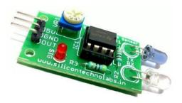
This device emits and/or detects infrared radiation to sense a particular phase in the environment. Thermal radiation is emitted by all the objects in the infrared spectrum and the sensor detects this type of radiation which is not visible to human eye.
