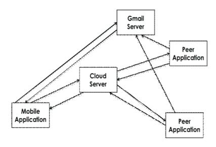
The Cloud's push to device messaging feature allows the request to be transferred to the peer's when they become connected to the internet.
