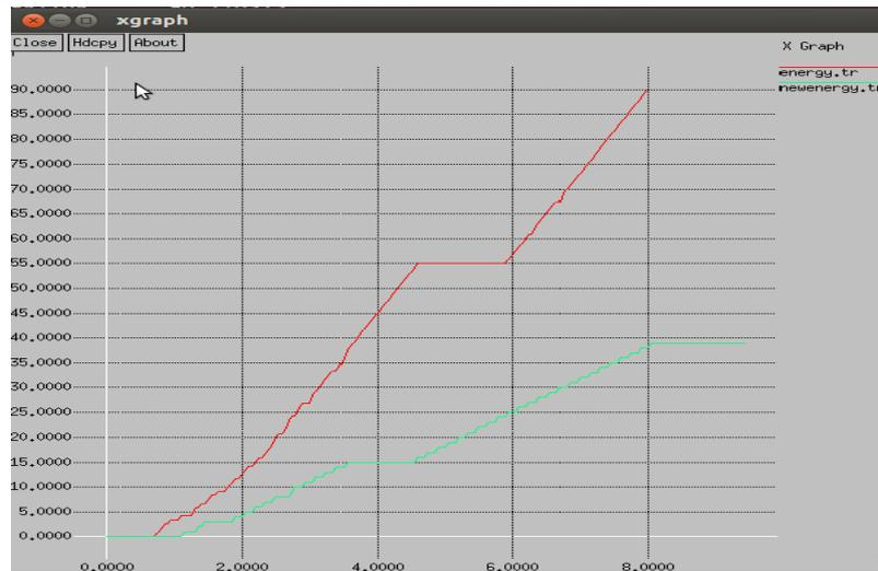
**Fig10:** Comparison of energy consumption for AODV and R-optimal algorithm in highway scenario
