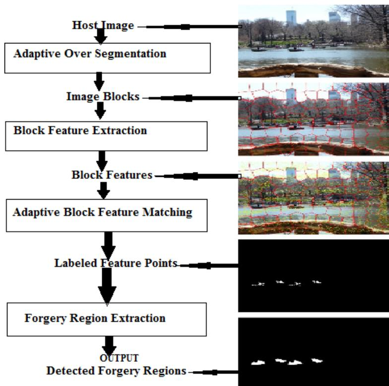
**Fig.1.** Copy-Move forgery detection scheme
