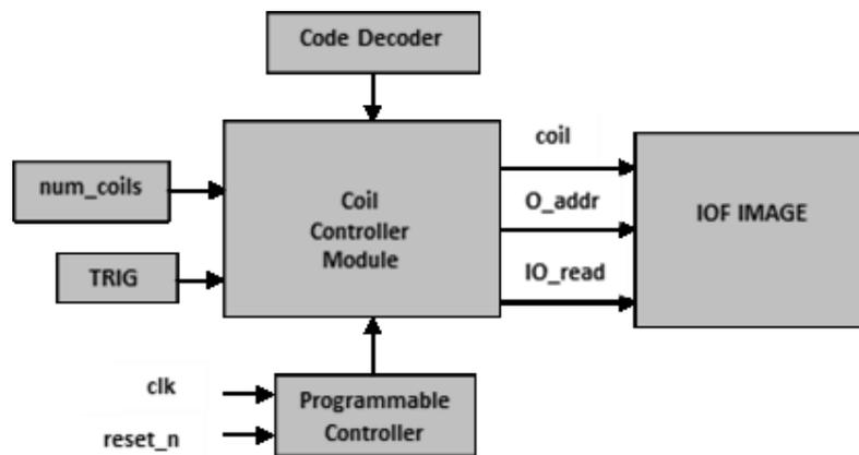
**Figure 5** Processing Blocks of Coil Control Operation
