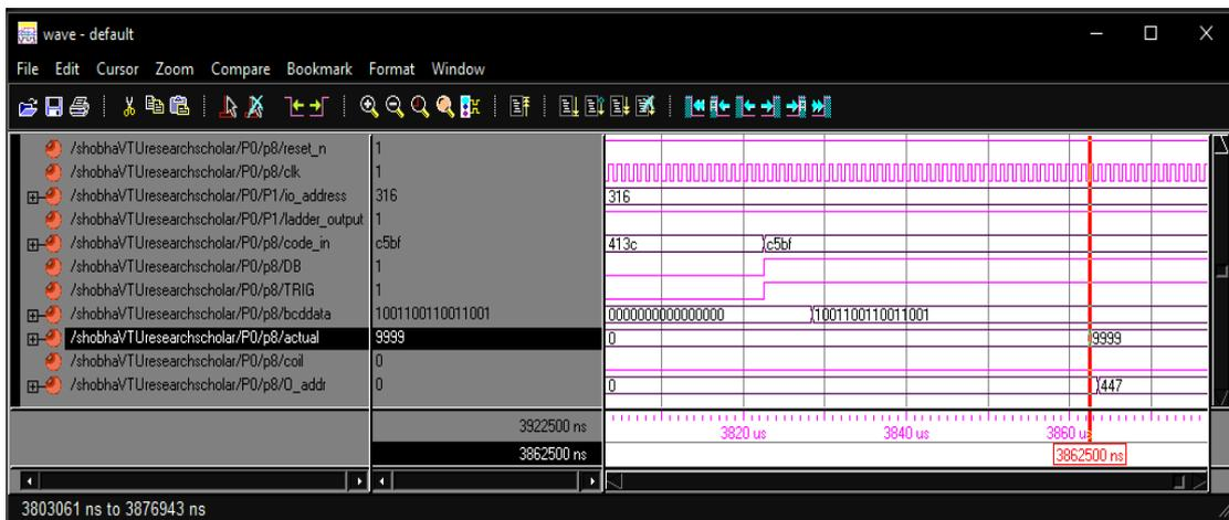
Figure 7 Simulated Waveforms for BCD to Binary Conversion Operation
