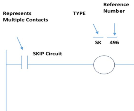
Fig. 2: Ladder Logic for Skip operation
