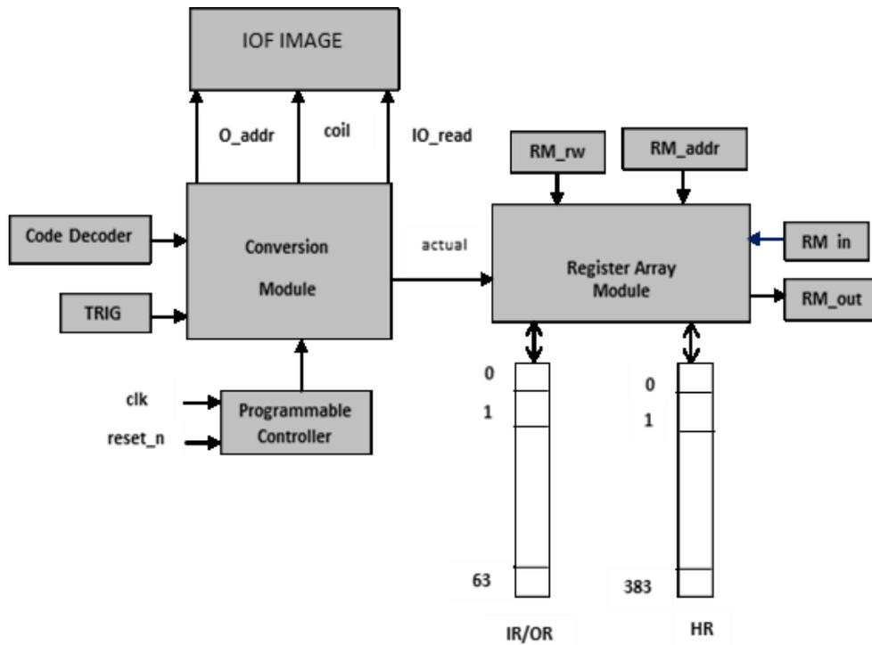
**Figure 4** Processing Blocks of Conversion operation
