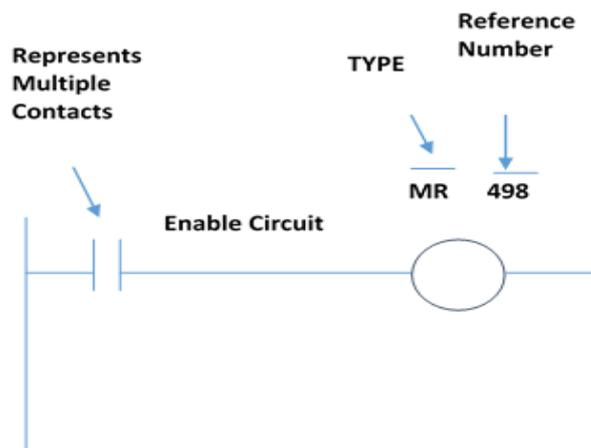
Fig. 3: Ladder Logic for MCR operation
