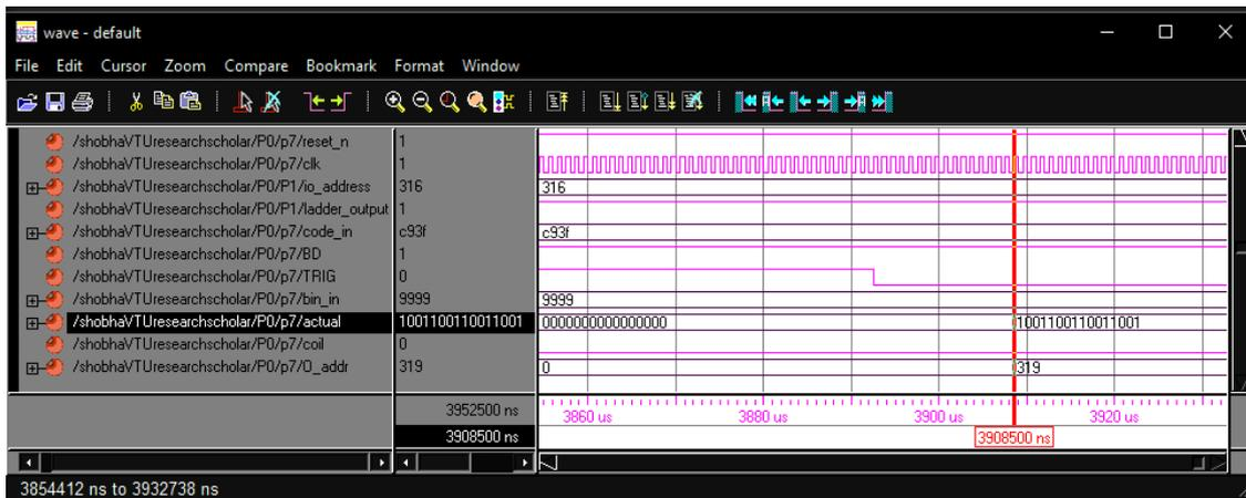
Figure 8 Simulated Waveforms for Binary to BCD Conversion Operation
