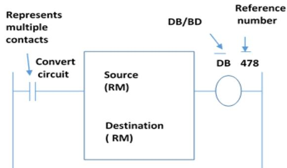
Fig.1: Ladder Logic for Conversion operation
