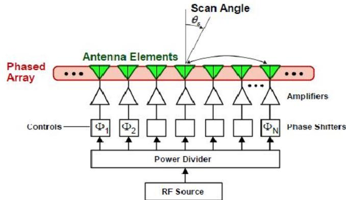
Figure 2: Phased array consisting N array elements.
