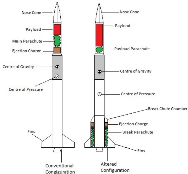
**Fig. 1:** Side view of the two rocket designs.
