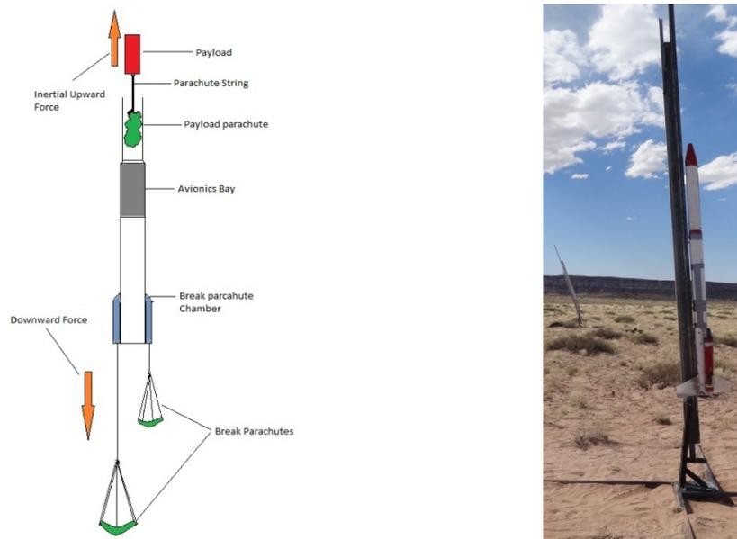
**Fig. 2:** (Right)Description of the recovery system deployment, (Left) Rocket with the new recovery system at the launch rail.
