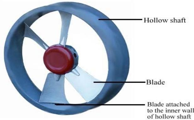
**Fig. 1:** Architecture Cut Section of Shaft Showing Circumferentially Fixed FAN (Designed Using CAD Software CATIA)
