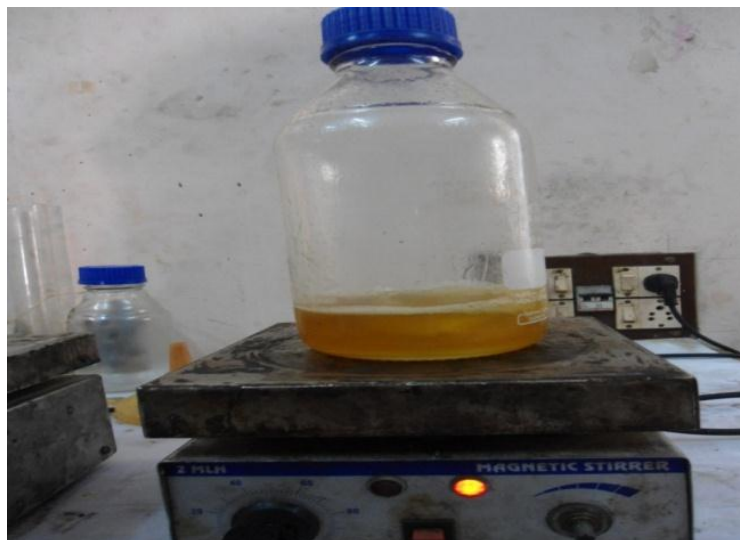
Figure 4: A sample of diesel and biodiesel mixed with catalyst in magnetic stirrer
