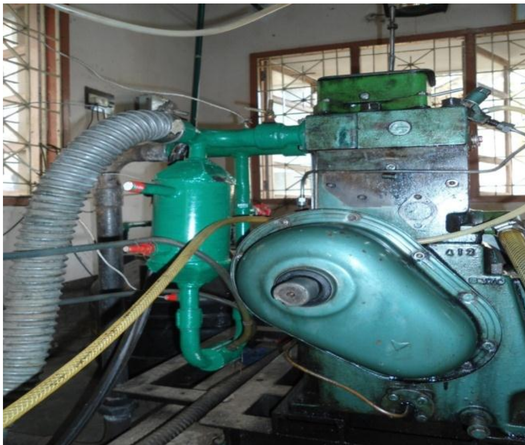
Figure 7: A schematic view of TV I Engine with Hot EGR
