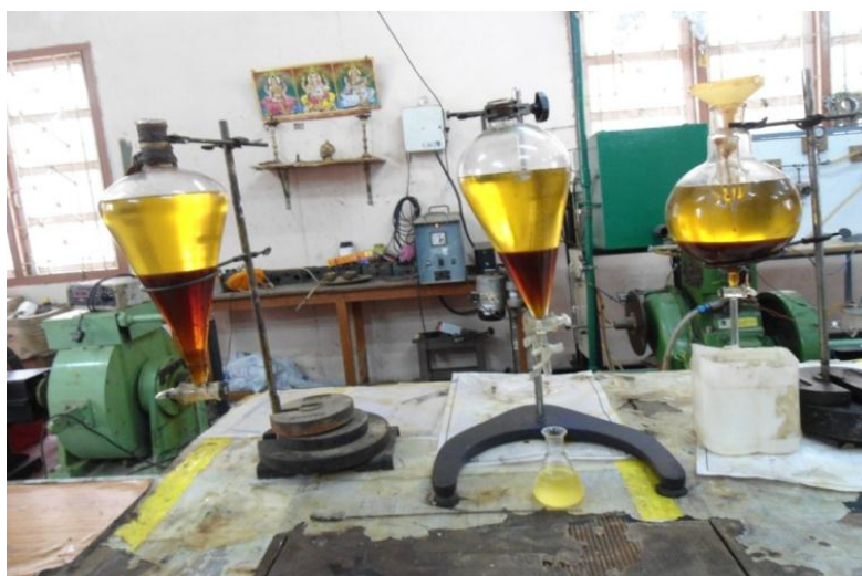
Figure 5: Separation of biodiesel and glycerol
